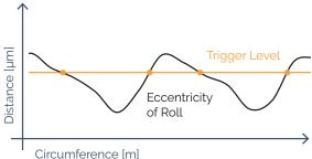
Positioned in the middle of the distance variations, the distance sensor triggers the measurement and image acquisition. This means that the focus for the optics is always at the correct distance. Aligned by an integrated, motorized movement, the sensor automatically adjusts to varying strip thicknesses.
