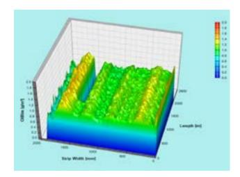
Dry streaks and incorrect lubrication is visible directly within the visualization.
